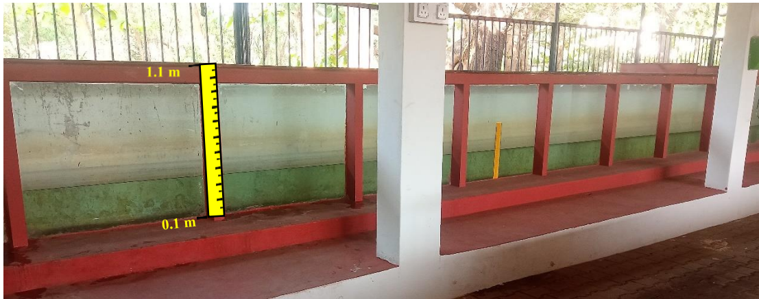
Figure 3.1 Side view of the two-dimensional wave flume
