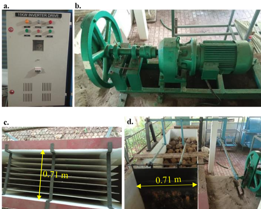
Figure 3.3 Wave generation system a) inverter drive, b) motor, c) wave filter and d) bottom hinged flap type wave paddle
