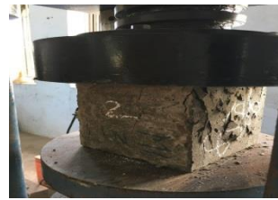
Figure 6. Test for Compressive strength
