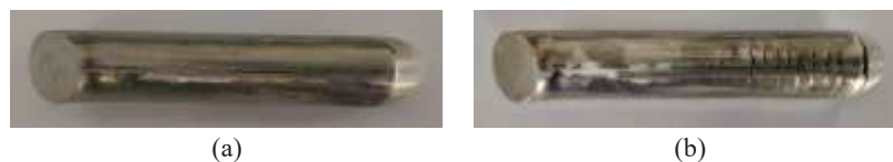
FIGURE 2. Al-10Zn-2Mg alloy ECAP processed at 150 °C (a) 1 pass and (b) 2 pass
