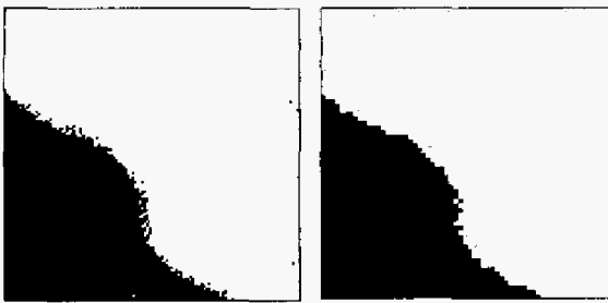
Fig. 8. Texture segmentation using HMM-Contourlet HMT method (a) 2x2 block (b) 4x4 block.
